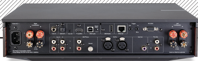
ABOVE: Switchable A/B speaker binding posts and pre/sub outputs (on RCAs) are joined by MM phono and three line ins (one balanced on XLR). Streaming is offered via wired/wireless Ethernet and BT aptX HD, with digital ins on optical (to 96kHz), coaxial (to 192kHz), USB-A/USB-B ports (to 768kHz and DSD512) and HDMI eARC (to 192kHz)
